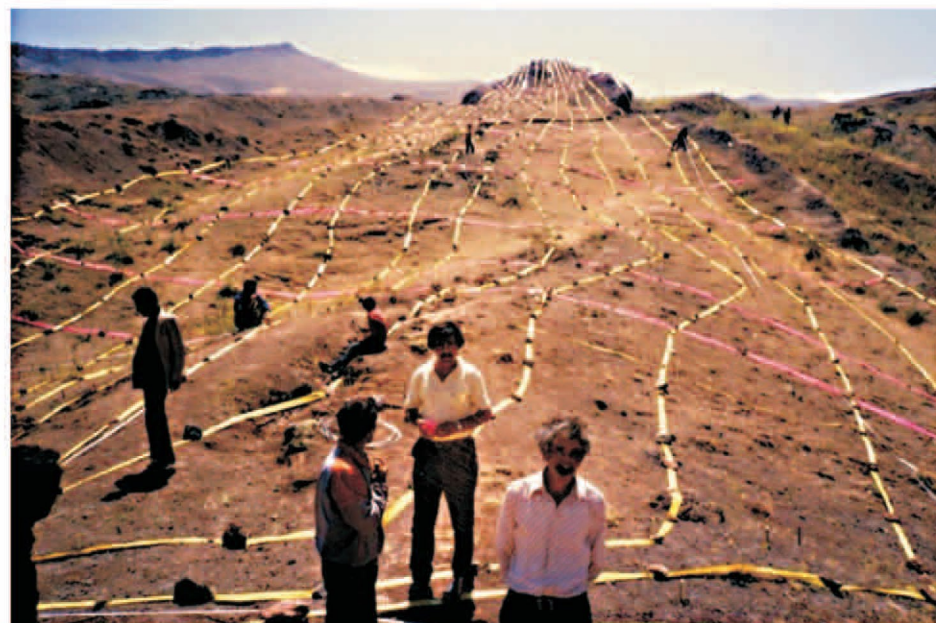
Iron Lines - Colored tapes laid along metal detector readings show a regular pattern of iron, further confirmation that the site contains the remains of an enormous man-made structure
